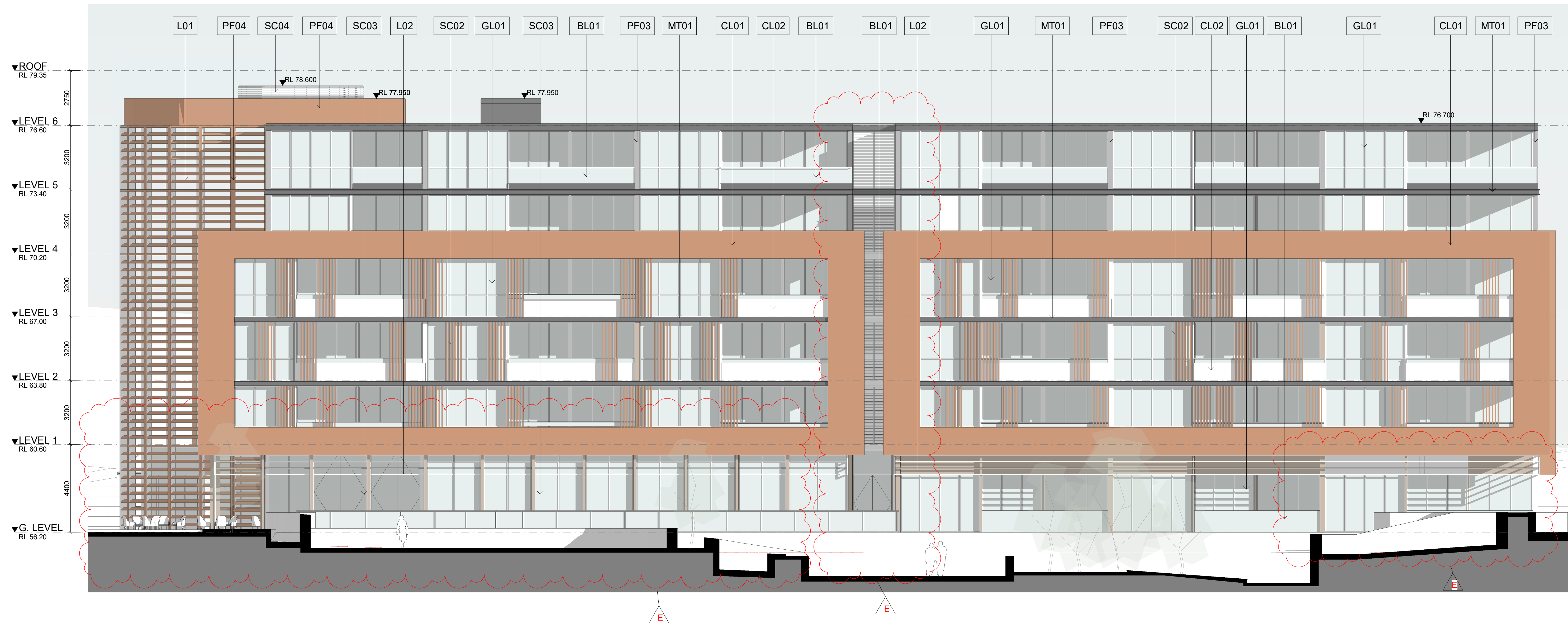
1 BUILDING E - EAST ELEVATION DA2.02 1 : 100
